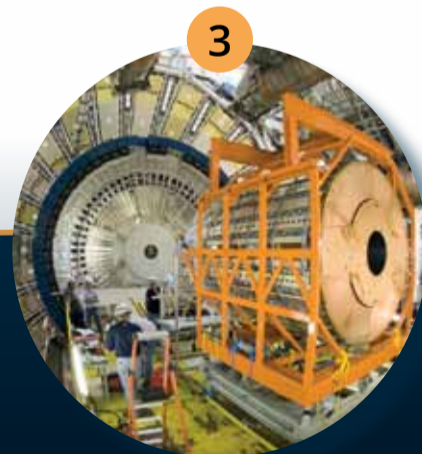
Inner Detector measures the momentum of each charged particle
